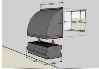
These are standard sizes in mm. Covers can be placed directly next to each other, and therefore are suitable for any type of air inlet.
