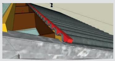
4. Apply insulation foam to the correct place: this should be above the purlin!
