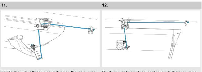
Guide the poly ethylene cord through the arm, rope guide roller and wire clamp
