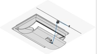
Mount the rope guide on the ceiling by using the stainless roundhead screws (5 x 60 mm)
