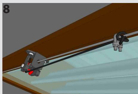
E: Fix the rope and wire with wire clamp
