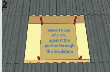
E: Make 4 holes of 2cm through the insulation
