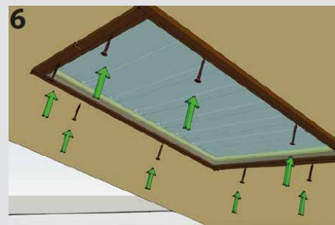
E: Fix polycarbonate window with 4 screws
