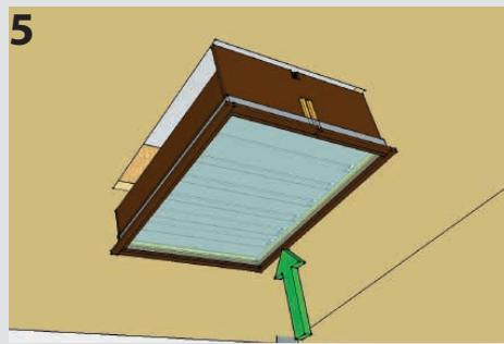
E: Place the black out roof window, fix with screws
